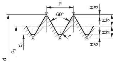
$$\begin{aligned}H &= 0,86603P \\h_3 &= 0,61343P \\d_2 &= d - (0,6495P) \\d_3 &= d - (2h_3) \\r &= \frac{H}{6} = 0,14434P\end{aligned}$$
