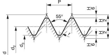
$$\begin{aligned}H &= 0,96049P \\h_3 &= 0,64033P \\d_2 &= d - h_3 \\d_3 &= d - (2h_3) \\r &= 0,13733P\end{aligned}$$
