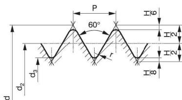
$$\begin{aligned}H &= 0,86603P \\h_3 &= 0,61343P \\d_2 &= d - (0,6495P) \\d_3 &= d - (2h_3) \\r_1 &= 0,10825P \\r_2 &= 0,14443P\end{aligned}$$
