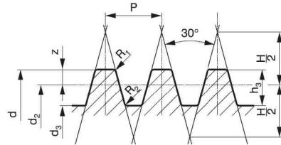
$$\begin{aligned}H &= 1,866P \\h_3 &= 0,5P + b \\z &= 0,25P \\d_3 &= d - (2h_3) \\d_2 &= D_2 = d - 2z\end{aligned}$$
