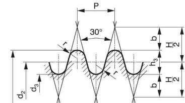
$$\begin{aligned}H &= 1,86603P \\h_3 &= 0,5P \\d_2 &= d - h_3 \\d_3 &= d - (2h_3) \\r &= 0,23851P \\b &= 0,68301P\end{aligned}$$
