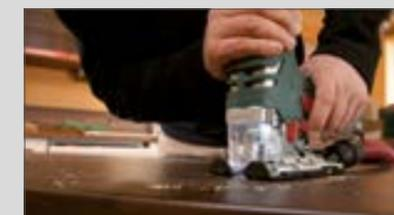
**Adjustable pendulum stroke**
