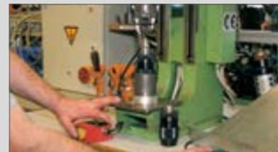
After assembly, each chuck is checked thoroughly for concentric operation and functional safety.
