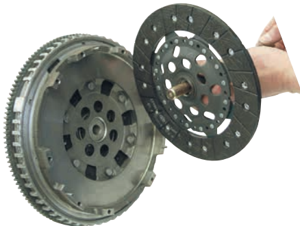
13. Insert clutch aligner and clutch disc into flywheel. Tighten clutch aligner.
