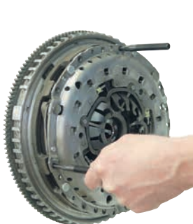
4. Remove knurled nuts and clutch pre-compressor. Remove clutch aligner and threaded bolts.
