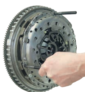
17. Remove knurled nuts, clutch pre-compressor and threaded bolts. Remove clutch aligner.
