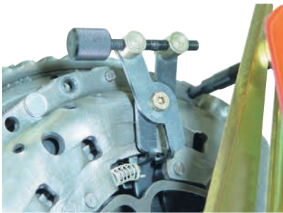
10. Insert reset tool. Turn back adjuster ring.
