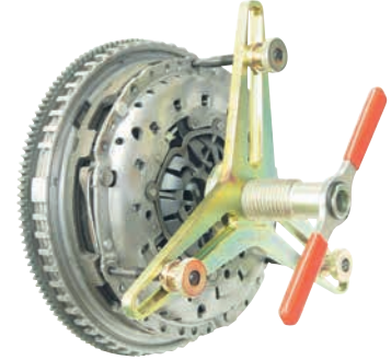
9. Compress diaphragm spring.
