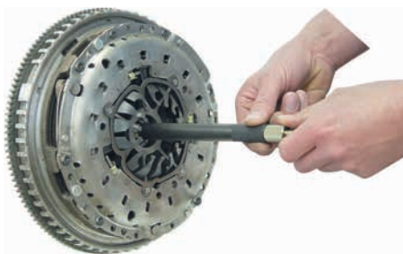
1. Insert clutch aligner into clutch and tighten it.
