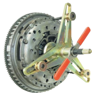
3. Compress diaphragm spring. Unscrew remaining fastening screws. Release pressure on diaphragm spring.
