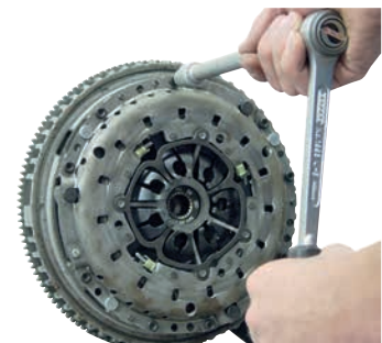
18. Screw in and tighten down the clutch pressure plate fastening screws.
