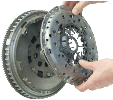
7. Install clutch pressure plate without clutch disc.
