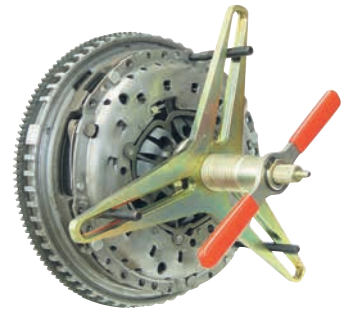
15. Screw down threaded bolts. Mount clutch pre-compressor.
